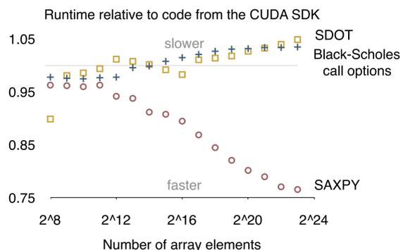
New and existing benchmarks were run to evaluate the effectiveness of the optimizations. The test system had a 512 MB NVIDIA GeForce 8800 GT GPU and CUDA 3.2.
