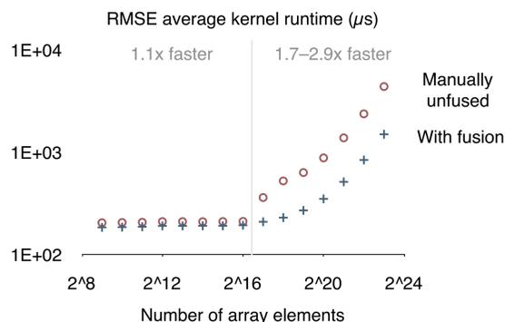
Array fusion is always performed by the Barracuda compiler; the test kernel was manually unfused to measure the impact of the simple fusion scheme.
