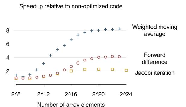
Three stencil kernels were compiled with and without on-chip memory optimization. Using on-chip memory gives dramatic speedups—8x for the weighted moving average.
